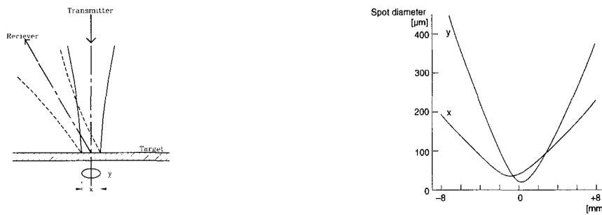
Fig. 5. Spot diameter according to the distance from the center of the measuring range.
