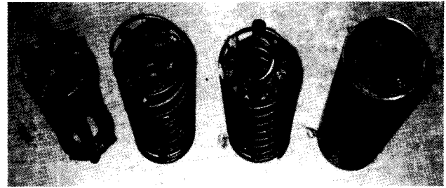
Fig. 5 Types of reinforcement in the fixed zone(From left side, no reinforcement, reinforced outside spiral, reinforced inside + outside spiral, steel pipe reinforced)
