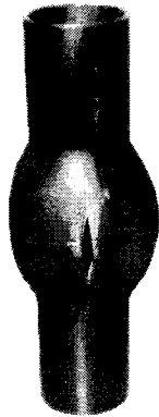
Fig. 19 Bursting during expansion
