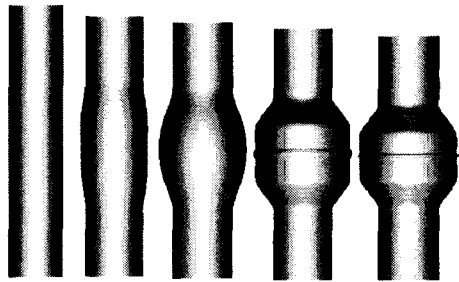
(c) Excessive volume of liquid in the tube
