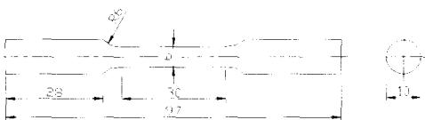
Fig. 1 Configuration of test specimen
