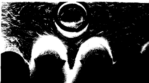
Fig. 6 Visualization photograph of coolant flow around spark plug and exhaust valve bridge
