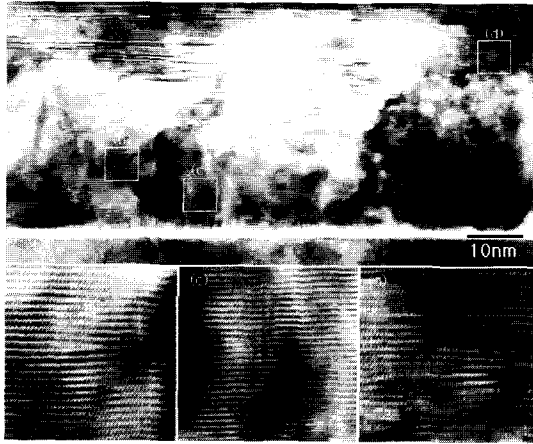
Fig. 1. High resolution TEM images of GaN/LT-GaN/AlN(MOCVD)/Si specimen; (a) Overall image showing GaN/LT-GaN/AlN/Si structure, (b) Dislocation, (c) Coalescence boundary, (d) Lattice mismatch
