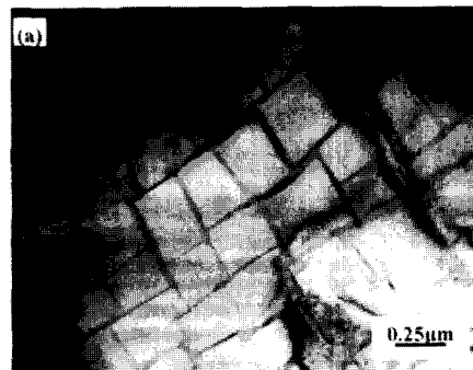
Fig. 1. The TEM observation of the microstructure on the surface of untreated IC6 surface.
