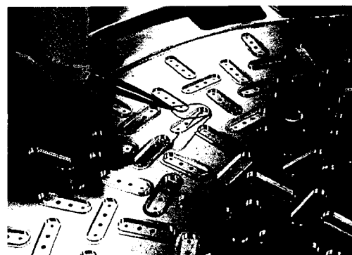
Fig. 9 Appearance of filler metal setting by spot welding before brazing
