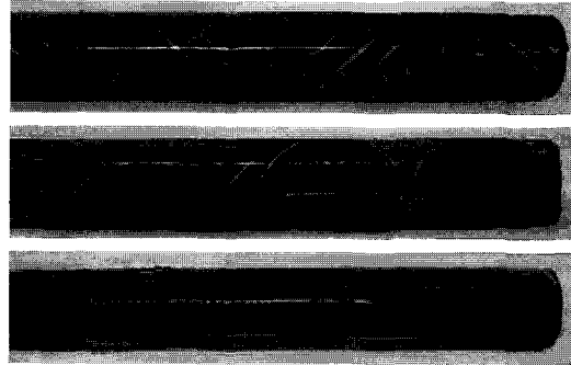
Fig. 8 Axial views for tracer mixing of Sulzer1, SSM1 and PPM1 model
