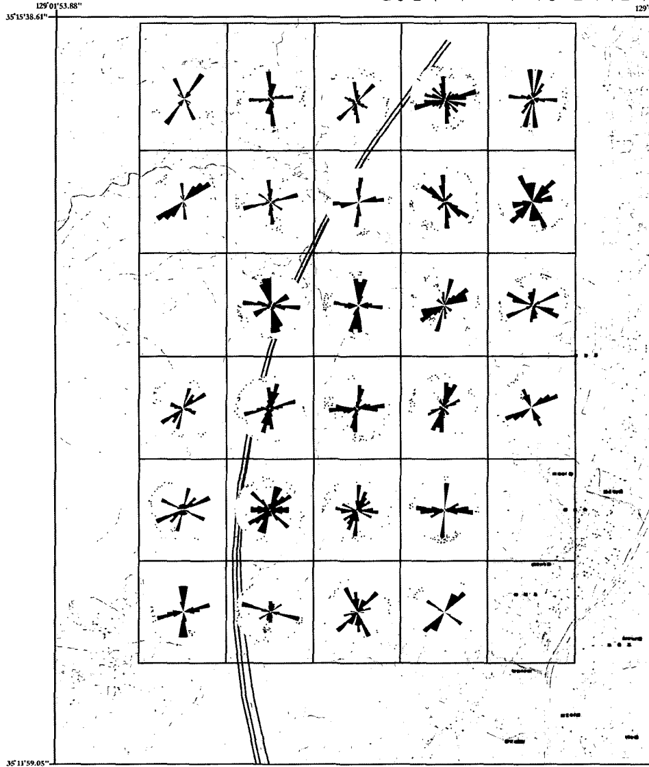
Fig 4. Rose and \pi -diagrams (equal-area and lower hemisphere) showing the attitudes of discontinuities (fractures) observed at each domain divided by 30 " \times 30 " area.
