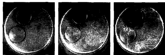
lift : 2 mm lift : 5 mm lift : 8 mm (c) Visualization result of D-type head]
