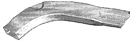
Fig. 1(b) CAD model to be hydroformed
