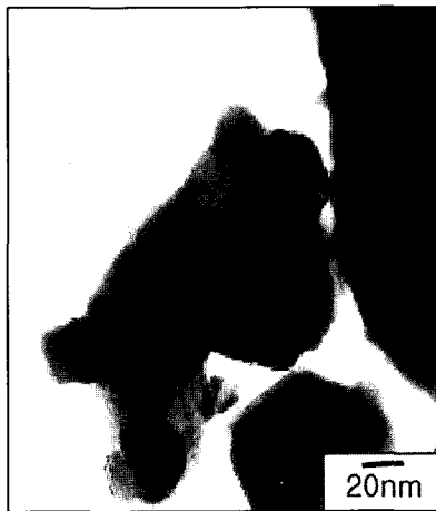
Fig. 3. TEM micrograph of nanostructured WC-Co-(TaC) 0.5 (VC) 0.5 powder carburized at 750°C for 2 hrs in flow CO atmosphere(TCP powder).
