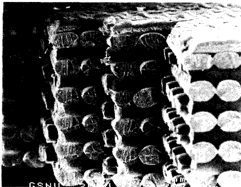
Fig. 7. Scanning Electron Microscope (SEM) picture of the fracture surface of a 45 degree specimen.
