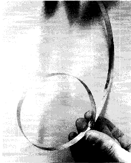
그림 2. Bi-axially textured Ni tape fabricated by a KAERI-powder process.
