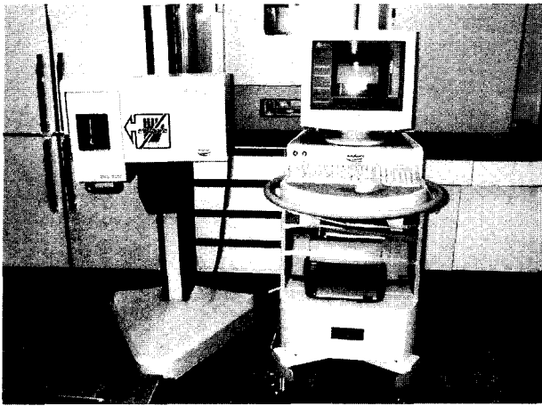
Fig 1. Infrared thermographic system.
