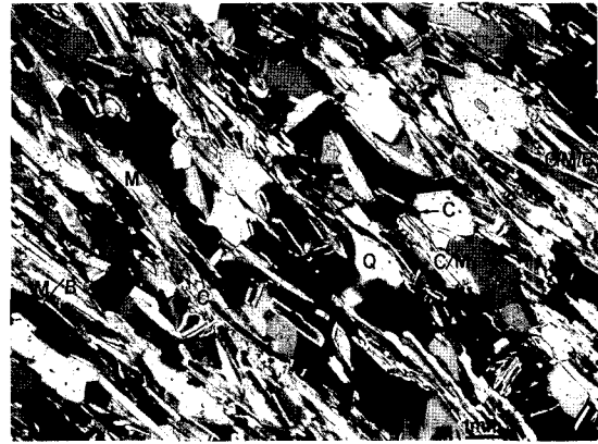
Fig. 2. A Polarized light photomicrograph (cross nicol) of a garnet zone metapelite from the Ogcheon Metamorphic Belt. The micas are oriented parallel to the cleavage running from the upper left to the lower right. The sample is cut perpendicular to the cleavage (foliation). The sample is composed of biotite (B; medium gray), muscovite (M; light gray), chlorite (C; dark gray) and quartz (Q; black, gray to white). The intergrowths between muscovite and biotite (M/B), chlorite and muscovite (C/M) and chlorite, muscovite and biotite (C/M/B) are commonly observed.
