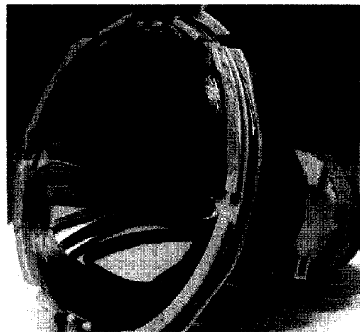
Fig. 5 Manufactured deflection yoke
