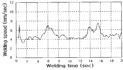
Fig. 11 Controlled welding speed ( From no gap to 0.4mm gap )
