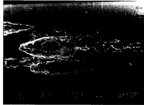
Fig. 8. SEM photograph showing pitting on sensor wire after anodic polarization test in synthetic ground water at 80°C.
