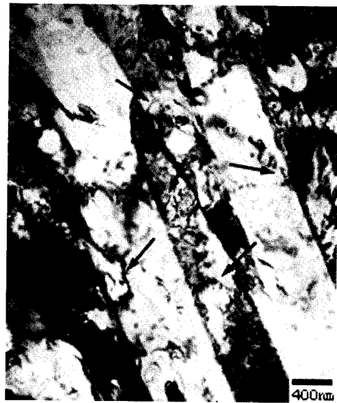
Fig. 3. TEM micrographs of water-quenched Zr-0.84Sn alloy after heat treatment at 990°C for 2 hrs.
