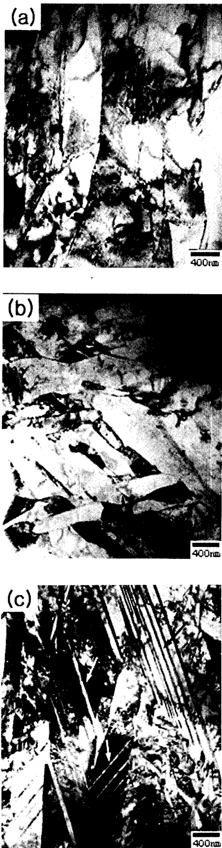
Fig. 4. TEM micrographs of water-quenched (a)Zr-0.84Sn-0.10V and (b)Zr-0.8Sn-0.19V and (c)Zr-0.86Sn-0.40V alloys after heat treatment at 990°C for 2 hrs.
