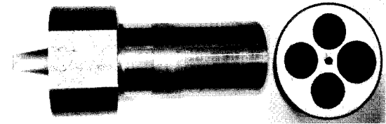
Fig. 7 The figure of rectangular conical plug and multihole container with difference of hole diameter
