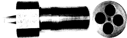
Fig. 6 The figure of rectangular conical plug and multihole container with no difference of hole diameter
