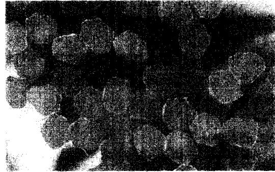
Figure 9. Cross section of PVA fiber prepared by wet spinning of PVA solution containing broic acid with an alkali coagulation bath.
