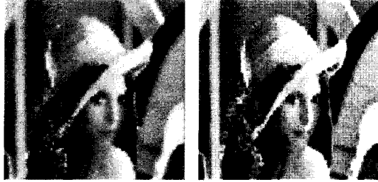
Fig. 9. Reconstructed Images Comparison (left : Condition 2-(c)(iter = 10^4 , RMSE = 18.35), right : non-iterative reconstruction method [3] (RMSE = 21.27))
