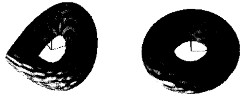
Fig. 12. A bump-mapped torus with a discontinuous texture function and with a periodized texture function
