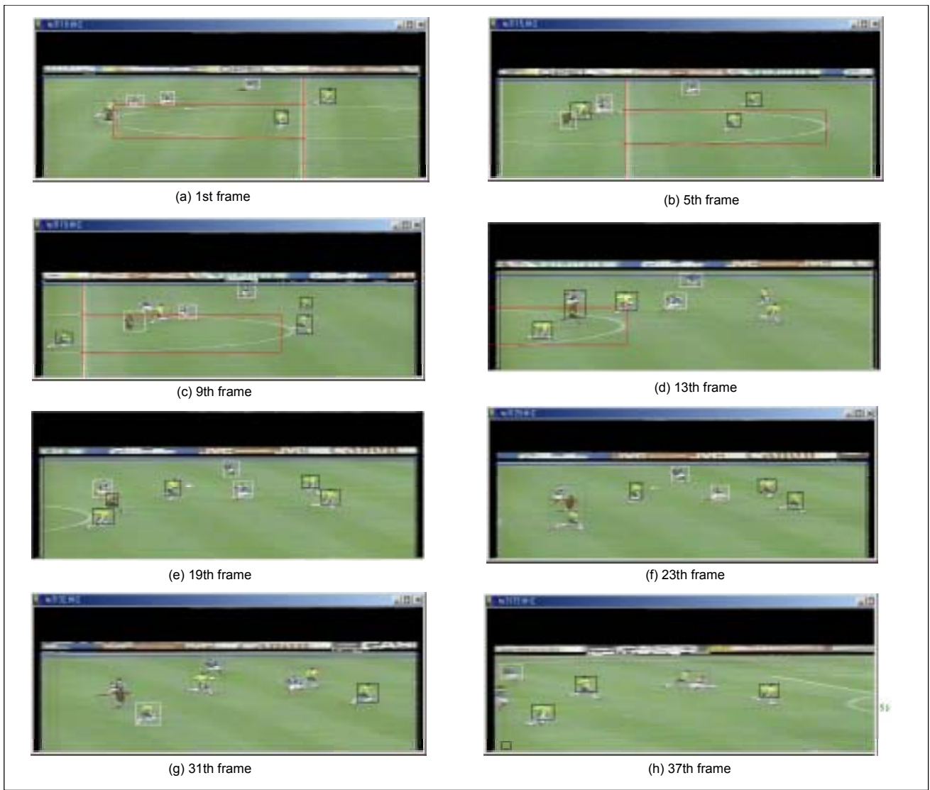
Fig. 14. The successive results of the player and line extraction algorithm.
