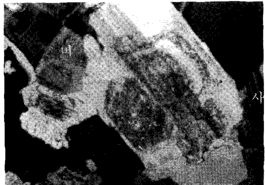
Fig. 2. Plagioclase show zonal structure which are partly sericitized. Myrmekite is developed around plagioclase.
