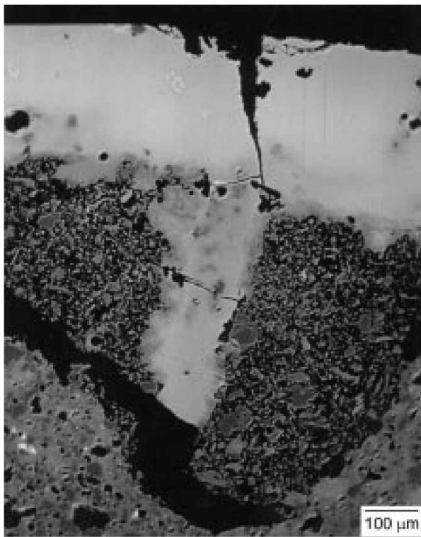
Figure 6. Backscattered electron images of white inlay in relation to glaze and body. (a) 19 (CH11-2); (b) 22 (CE11-3); (c) 166 (S-27-6).
