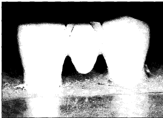
Fig. 5. Fracture pattern of all-ceramic fixed partial denture.
