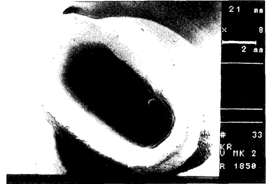
Fig. 10. SEM of poorer marginal fit by the CECEC ® In-Ceram crown (10x).
