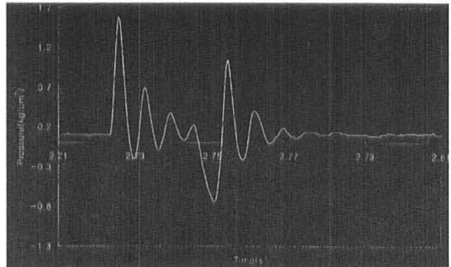
Fig. 4 Characteristic of the pressure distribution (Deadrise Angle 0^\circ , drop height : 50 \text{ cm} , sensor position : center)
