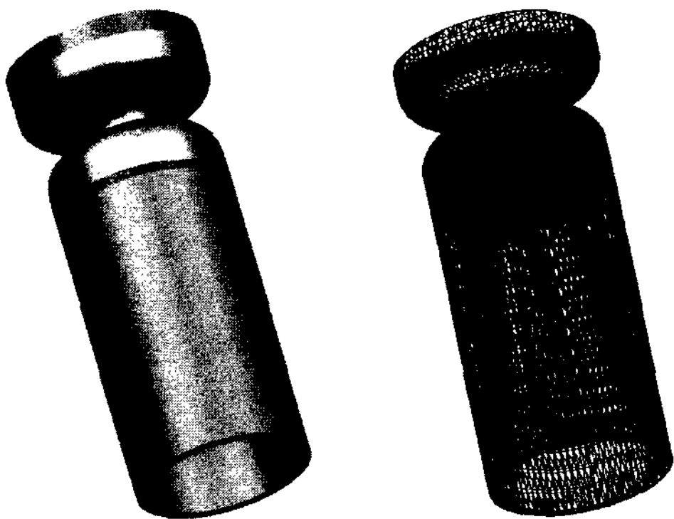
(a) 3D modeling for CATIA (b) STL file for geometry transfer
