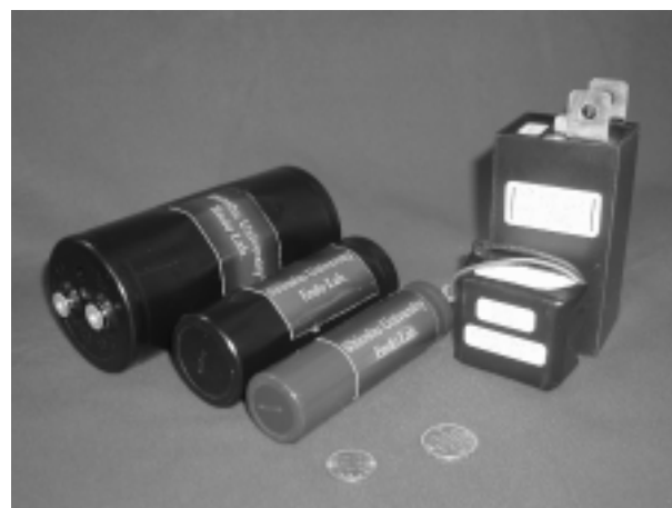
Fig. 19. High power capacitor of (left side of picture, cylindrical type) 1,500~4000F, working voltage is 2.5 V with non-aqueous solvent, (right side of picture, box type) and 25~90F, working voltage is 0.9V with aqueous electrolyte.
