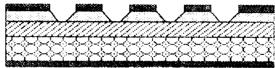
(b) Patterning of masking layer and anisotropic SCS wet etching
