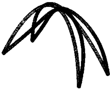
Fig.16. Second vibration mode (longitudinal sway)
