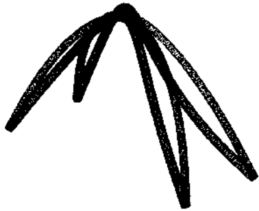
Fig.15. Buckling mode (twist)
