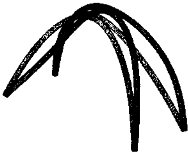
Fig.17. Third vibration mode (side sway)
