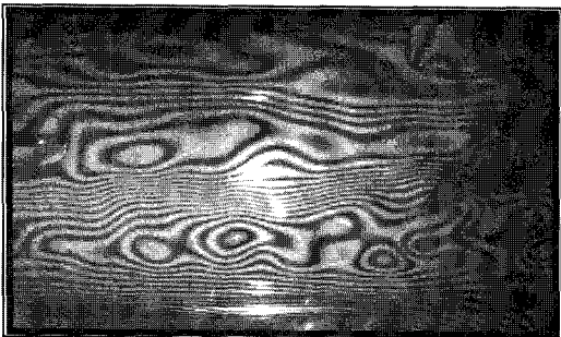
Fig. 7 The vibration mode at the delay time 150ms
