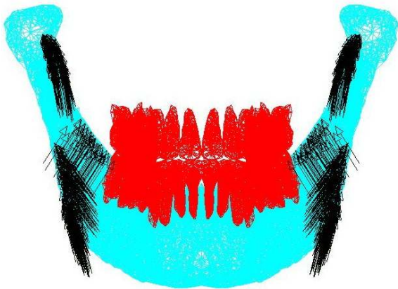
Fig. 1. Loading condition of mandible during bilateral clenching
