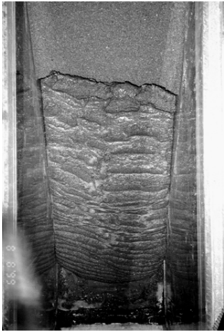
Fig. 7. Unreinforced embankment failure in sand (Dr=40%, 1:1.5, Fast rising)
