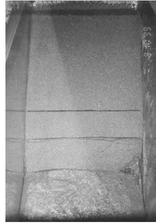
Fig. 8. Reinforced embankment failure in sand (Dr=40%, 1:1.5, Fast rising)
