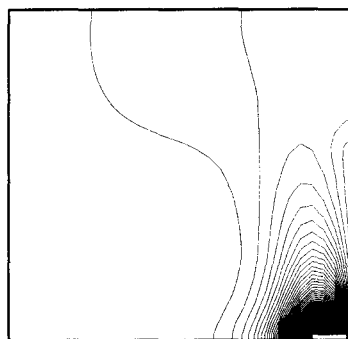
Fig. 5. Isotherms for different locations and sizes of outflow opening at vertical wall
