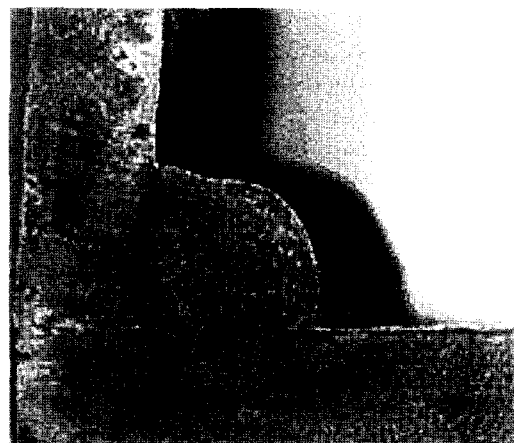
Fig.14 Weld bead with excess convexity obtained by welding conditions determined from neural network for desired bead shape( welding speed=4.2(mm/sec), arc voltage=21(V), welding current=200(A), gas flow rate=18(l/min), offset distance=0(mm) )
