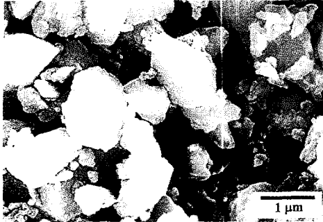
Figure 1. SEM micrograph of anisotropic magnetic Sr-ferrite powders.
