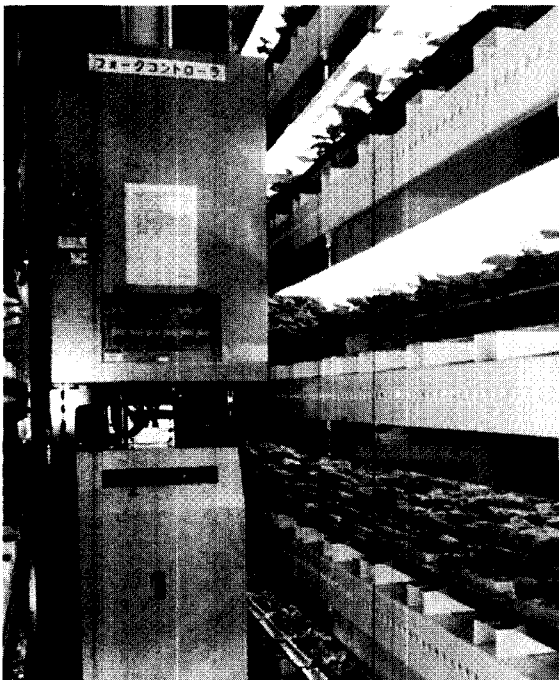
Figure 3. A tray transporter installed between the basic modules in each production room.
