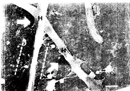
**Fig. 5.** Fungal slime (dotted line) and erosion trough (arrow) by enokitake hyphae. bar=2 $\mu$ m
