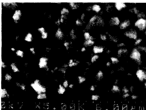
(c) t_{\text{off}} : 150\text{msec} , i_m : 2.0\text{A}/\text{dm}^2
