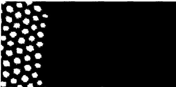
FIG. 2. The output sharp edge image of an image guide with average 4 \mu\text{m} diameter microfibers.
