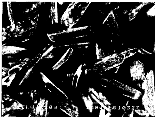
Fig. 17. Scanning electron micrographs of recrystallized gypsum.
