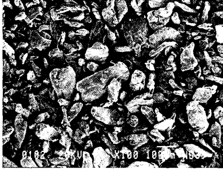
Fig. 1. SEM micrographs showing the raw Fe powder.
