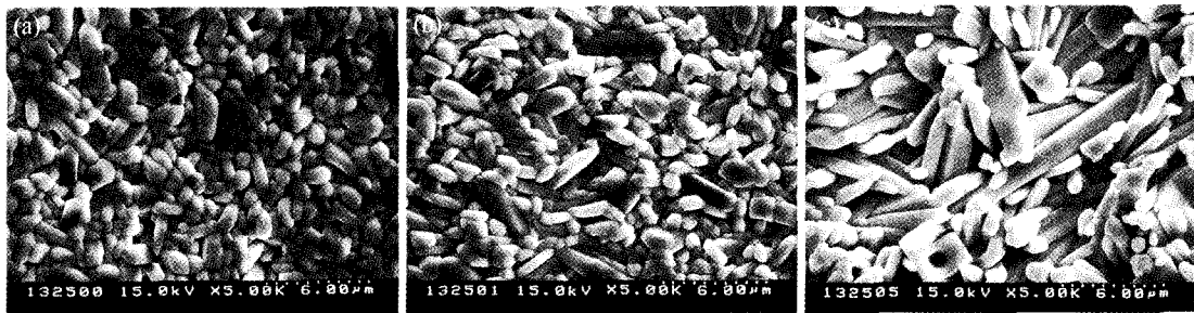
Fig. 3. SEM photographs of BPNT with different glass content sintered at 1350°C: (a) 0 wt%, (b) 1 wt% and (c) 3 wt%.
