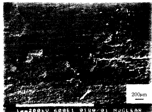
Photo. 2 Surface profile of corroded part of NW specimen after weight loss test of free corrosion condition (left : base metal, right : weld metal)
