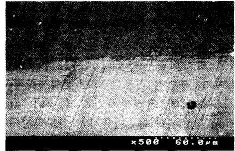
Fig. 16 SEM micrograph can be seen the micro crack near the interface
